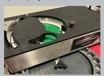
The Auto-Print® Oral Solid Feeder will dispense tablets up to ½" in diameter and can accommodate most available tablet and capsule medications. Packaging speed per minute is dependent on tablet or capsule size. This complementary attachment is available only on Auto-Print® models featuring a 9300 printer module. This option is not available on the Auto-Print® Express 90 model.
